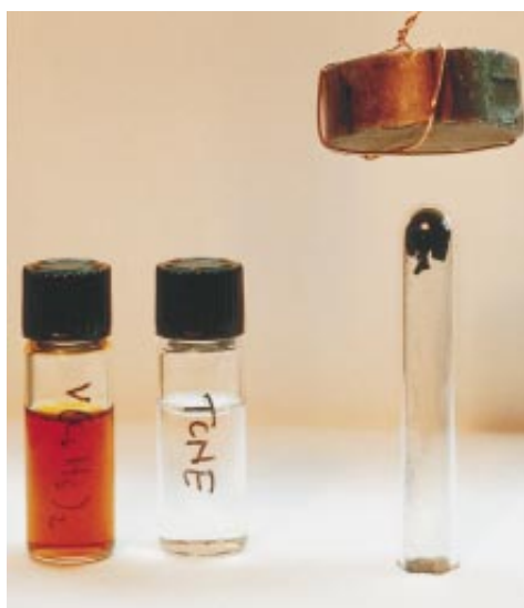
NONMETALLIC MAGNET (inside tube, at right) is made from the two liquids shown at the left.
